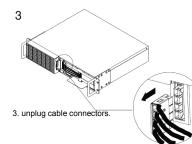
4. Pull out the old battery pack and replace new one Reassemble the retaining screws, covers, black and red cable, and front panel in the reverse sequence of the above steps. Recharge the unit for 4-8 hours to ensure maximum UPS battery runtime
