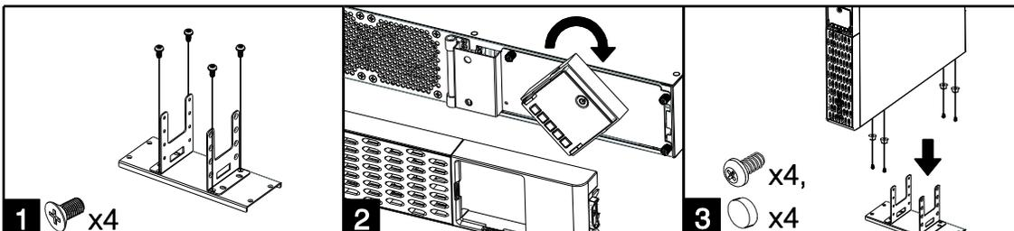
1. Attach the brackets to the baseplate with the provided M4 flat head screws.
