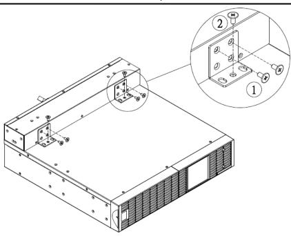
MBP mounted with a CyberPower UPS in rackmount mode
