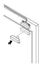
**NOTE:** The DOORSENSOR should be mounted on the opening end of the door (opposite side of the hinges).
