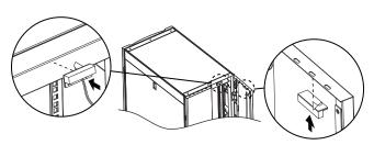
NOTE: The DOORSENSOR should be mounted on the opening end of the enclosure door (opposite side of the hinges). The magnet should be mounted flush against the inside edge of the door. Align the switch with the magnet mounted on the enclosure door and adhere it to the outside of the enclosure frame where the door closes.
