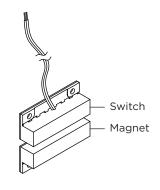
(1) Door Switch Sensor with 10ft (3m) Cable
