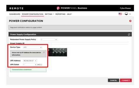
**11-3.** If the UPS does NOT have an RMCARD installed, set the IP address of a neighbor ESXi host server which has PPB VA Local installed and is powered by the same UPS (see below diagram).
