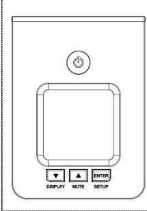
**Power On:** Press the POWER button for approximately 2 seconds and you will hear a short steady tone (1 second). Release the button after a short beep.
