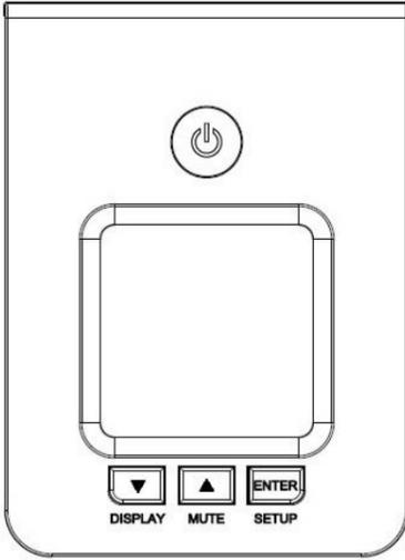
**Power On:** Press the POWER button for approximately 2 seconds and you will hear a short steady tone (1 second). Release the button after a short beep.
